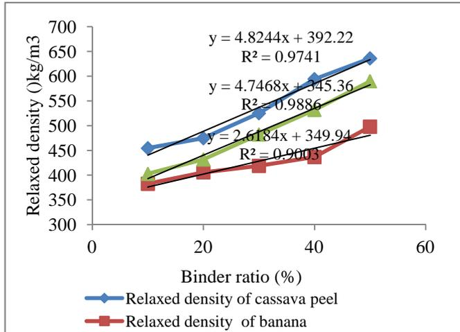
Fig. 3. Effect of binder ratio on relaxed density of briquettes
