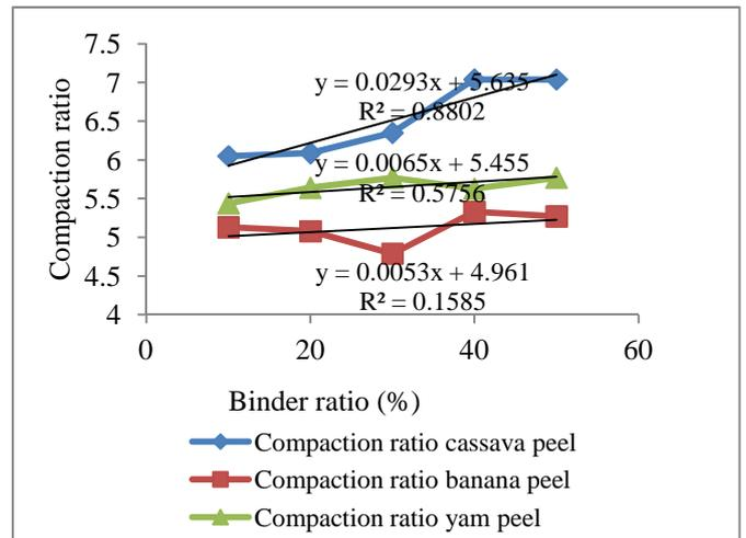
Fig. 4. Effect of binder ratio on compaction ratio of briquettes
