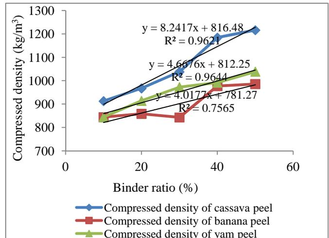
Fig. 2. Effect of binder ratio on compressed density of briquettes
