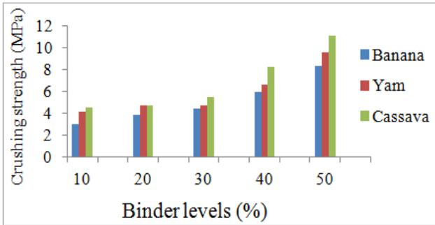
Fig. 7. Effect of binder levels on crushing strength of the water lettuce briquettes
