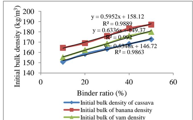
Fig. 1. Effect of binder ratio on water lettuce briquettes
