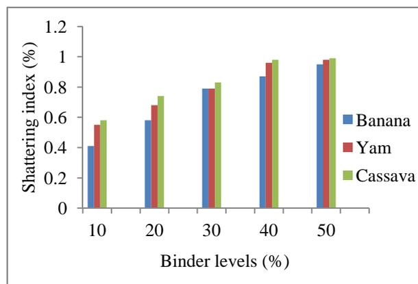
Fig. 6. Effect of binder levels and types on shattering index of water lettuce briquettes
