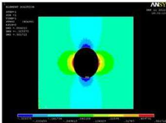
Figure 2. Tsai-wu failure index for UD-GFRP.
