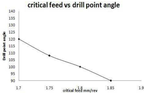
Figure 3. Effect of drill bit angle over critical feed rate for UD-GFRP.
