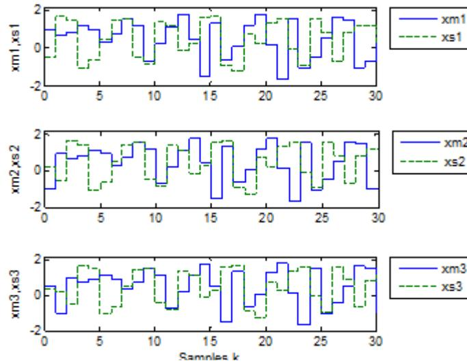
Fig. 3. Evolutions of the master and slave Hénon maps state responses when controller is switched off.
