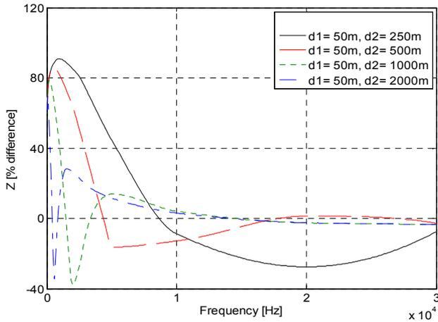
Fig. 1. Relative differences of ground return impedances against frequency for the structure "sedimentary rocks – granite – basalt".
