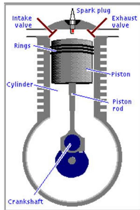
**Figure 3.** Basic IC engine diagram (Courtesy Wikipedia).
