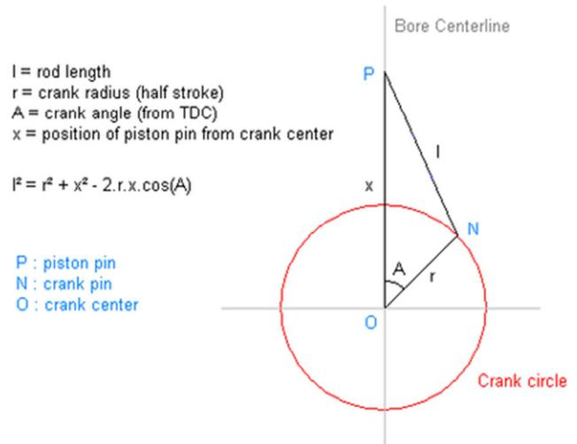
Figure 4. Crank Angle definitions (Courtesy Wikipedia).
