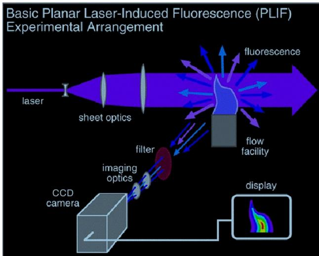
**Figure 2.** Laser Induced Fluorescence set-up (Courtesy- Velocimetry& Wikipedia).
