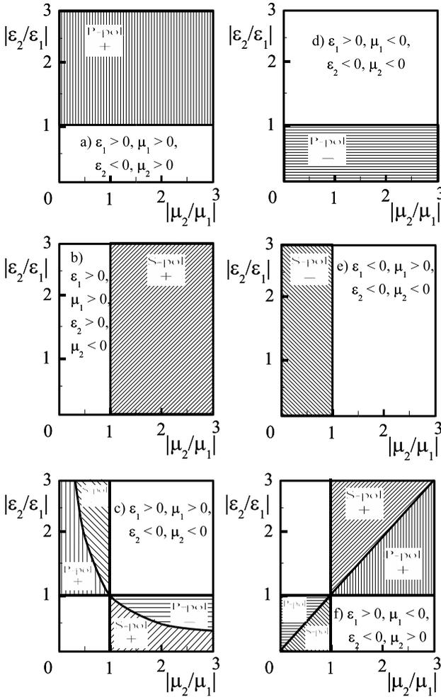
**Figure 7.8** The six cases of negative refractive interfaces that are possible between media with different  $\epsilon$  and  $\mu$ . The parameter ranges when the interfaces support surface modes and have negative refractive interface (shown by a - sign) or a positive refractive nature (shown by a + sign) are marked by different gray shades for P-polarized and S-polarized surface modes. No surface modes are possible in the white regions. Redrawn based on the data of Kats et al. (2007).
