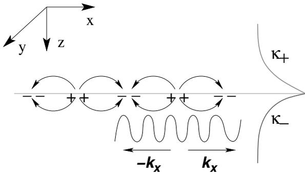
**Figure 7.1** Schematic representation of a surface plasmon at an interface between a negative and a positive dielectric medium, and the associated charge density fluctuations. The exponential decay of the fields normal to the surface and the propagating nature along the surface are depicted schematically. (Reproduced with permission from (Ramakrishna 2005). © 2005, Institute of Physics Publishing, U.K.)
