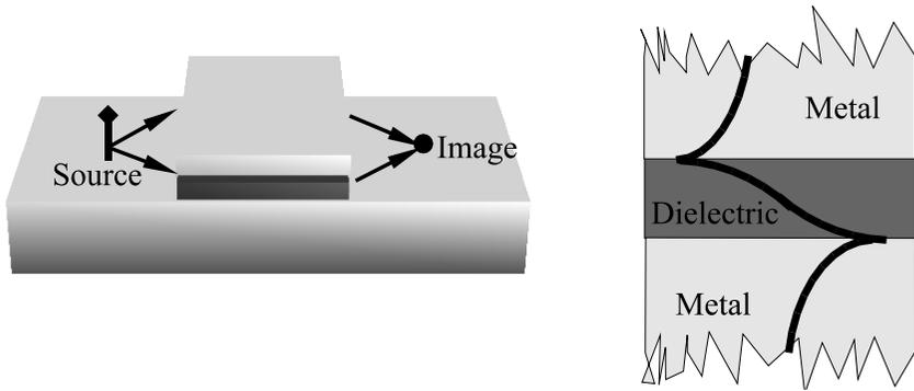
**Figure 7.9** A schematic picture of the negative refraction of surface plasmon modes on a metal surface by coupling to the slab modes of a heterostructure. Negative refraction is enabled when the slab modes, particularly the anti-symmetric modes, have anti-parallel energy flow and wave-vector (shown on the right). The heterostructure acts as a flat lens focusing a point source placed on one side.
