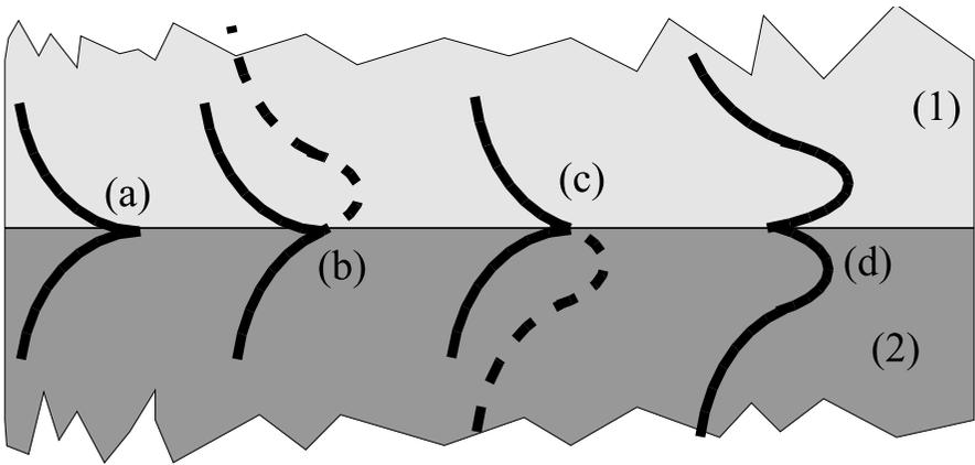
**Figure 7.11** An interface between two media (1) and (2) can support a variety of surface waves, which are shown schematically: (a) Both media are linear. (b) Medium (1) is linear while medium (2) is nonlinear. (c) Medium (2) is linear while medium (1) is nonlinear. (d) Both media are nonlinear. The dashed line corresponds to the continuation of the sech solution into the other medium and peaks at the location of the displaced center of the solitonic solution ( $z'$ ).
