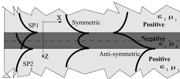
**Figure 7.3** Schematic representation of the geometry of the slab of a material with negative  $\epsilon$  or  $\mu$ . The surface plasmons on two interfaces are no longer independent and get coupled to give rise to coupled slab plasmon polariton excitations. The slab modes can have field distributions that are either symmetric or anti-symmetric with respect to the center of the slab.
