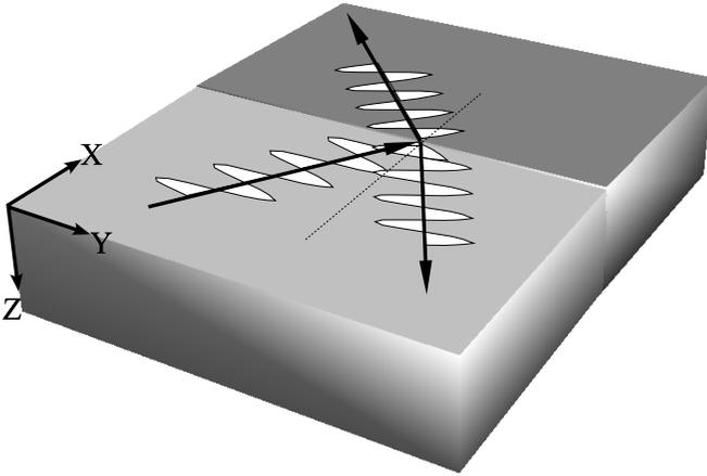
**Figure 7.7** A schematic picture of surface plasmon modes at the surfaces of two media (shown by different shades of gray). The surface waves can undergo negative refraction at the interface between the two surfaces (media) as shown depending on the material parameters of the two media.
